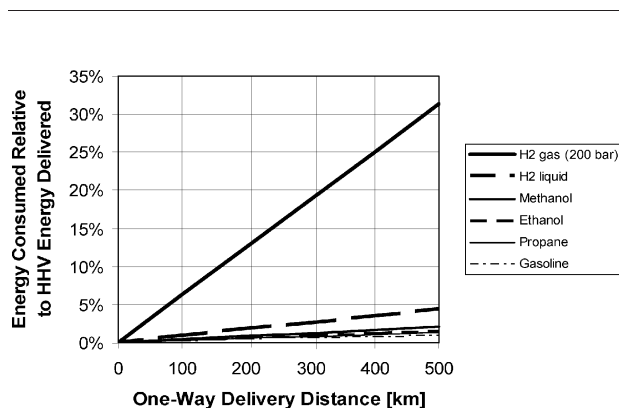
Fig. 6. Energy needed for the road delivery of fuels relative to their HHV energy content.
